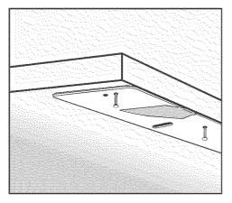
• **Center** the steam deflector in the opening for the dishwasher and align with the lower front edge of the countertop.
